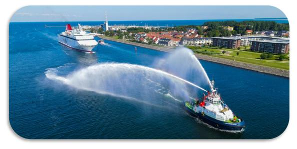
Pictured: Boluda's tug 'VB Bremen', a Voith-Schneider driven harbour and seagoing tug with 60 tonnes bollard pull, welcomed and escorted the ferry 'Hansa Destinations' of AB Gotland on its maiden voyage from Stockholm to Rostock on August 31<sup>st</sup> 2021.
